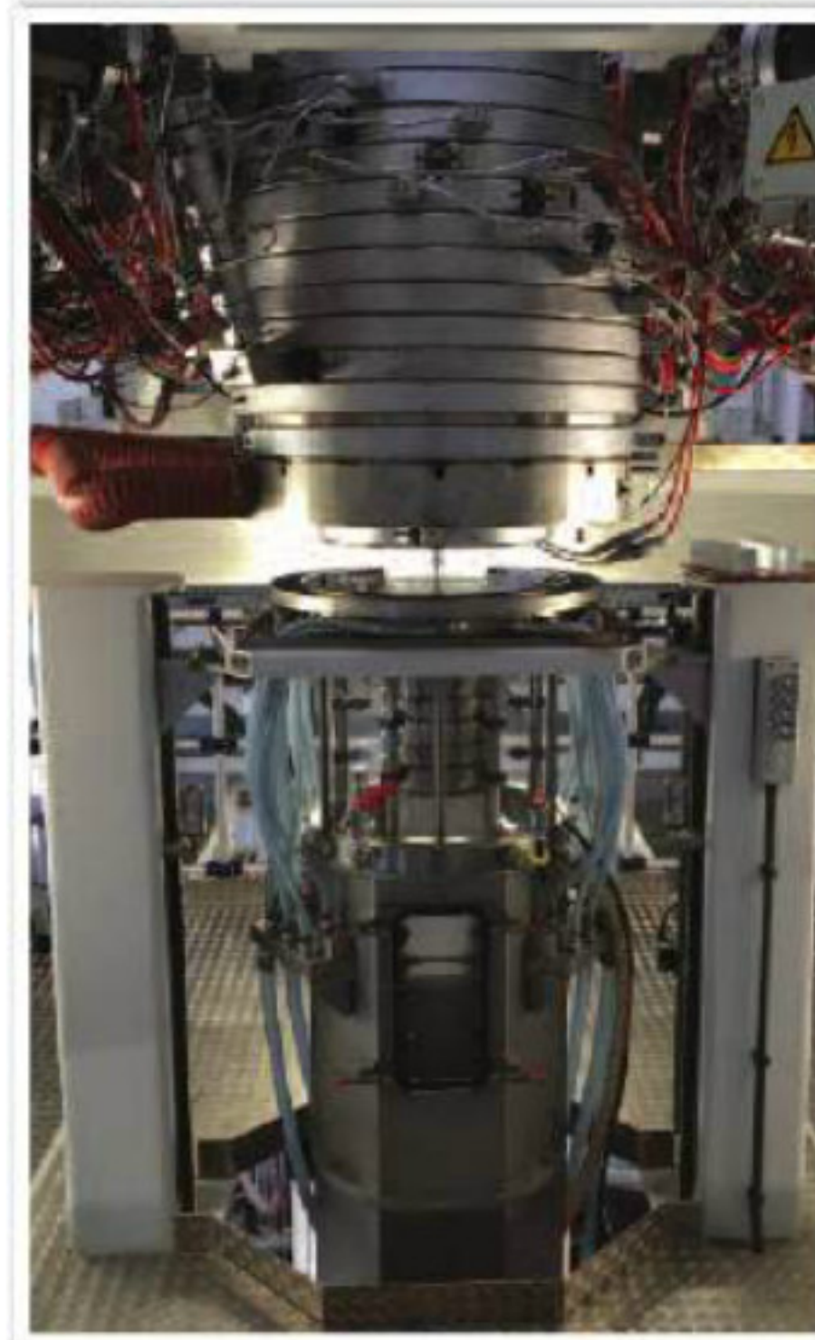
Kuhne's latest die design is the 13-layer Mo-Con (Modular Concept stackable die)
